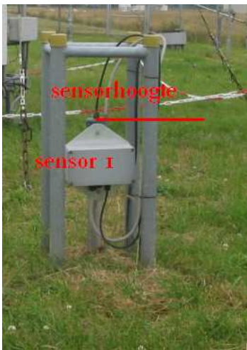
Figure 4: Piezometer sensor at the CESAR observatory, Cabauw. Photograph courtesy of Mariska Konging, KNMI.
